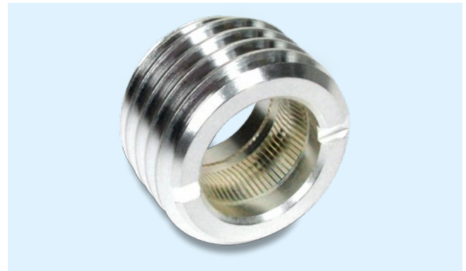
Special termination using standard ODU LAMELLA \varnothing 22 mm in special carrier for high-performance securing: – Nominal current approx. 550 A
