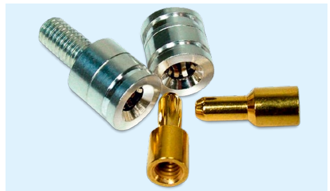
Application in the automotive sector: – Special lamella with radial compensation ( \pm 0.3 mm) – Nominal current 25 A – Vibration-resistant – Application temperature -40^{\circ}\text{C} to +125^{\circ}\text{C} , briefly +170^{\circ}\text{C}
